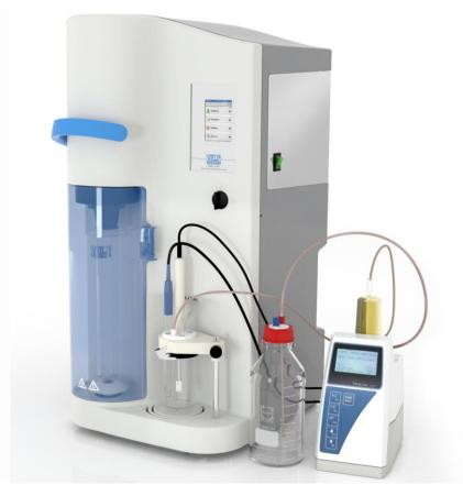
The UDK 149 Automatic Distillation Unit is designed to perform nitrogen and protein content analysis according to the Kjeldahl Method (TKN) in the Food & Feed industries and several other applications in environmental control (phenols, nitrogen in water, sludge, soil and lubricant) and also in the chemical and pharmaceutical industries after having digested the sample accurately.
